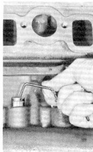
Lifting Tappet With C-3216 "Grappling" Hook
